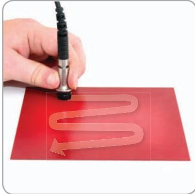
When the Scan Mode\* is selected users can slide the Scan probe over the entire surface area. As the probe is lifted off the surface the gauge displays the average coating thickness value, the highest thickness and the lowest thickness values. Each set of three readings (average, high and low) can be displayed on the run graph and stored into the memory.
