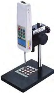
SPF Keystroke Test Stand
