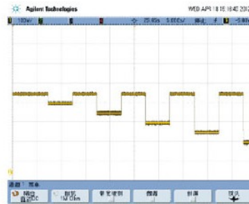
ISO 16750-2 voltage drop rest experiment
