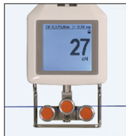
Depending on the measuring position the LCD display automatically rotates in 90° steps
