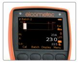
During a scan the live reading together with an analogue bar graph is displayed
